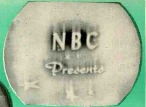
Fig. 2—Vertical picture bounce.
