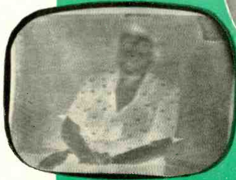
Fig. 1—Negative picture on screen.
